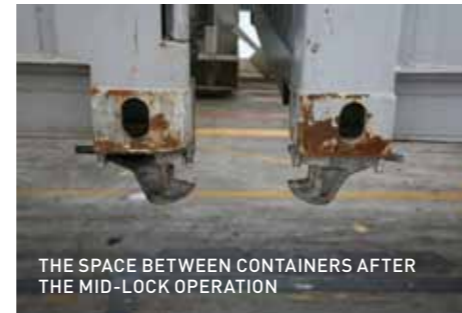
THE DIFFERENCE BETWEEN CONVENTIONAL & MID-LOCK TWIST-LOCKS
